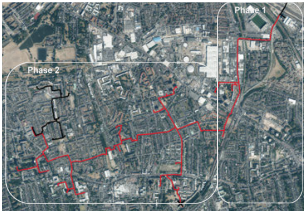
Figure 3. District Heating Network Expansion towards North Peckham
